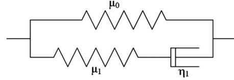
FIG. 8. Representation of a standard linear solid model. It consists of a single-spring element ( $\mu_0$ ) in parallel connection with a Maxwell model. The Maxwell model consists of another spring element ( $\mu_1$ ) in series connection to a dashpot element ( $\eta_1$ ).
