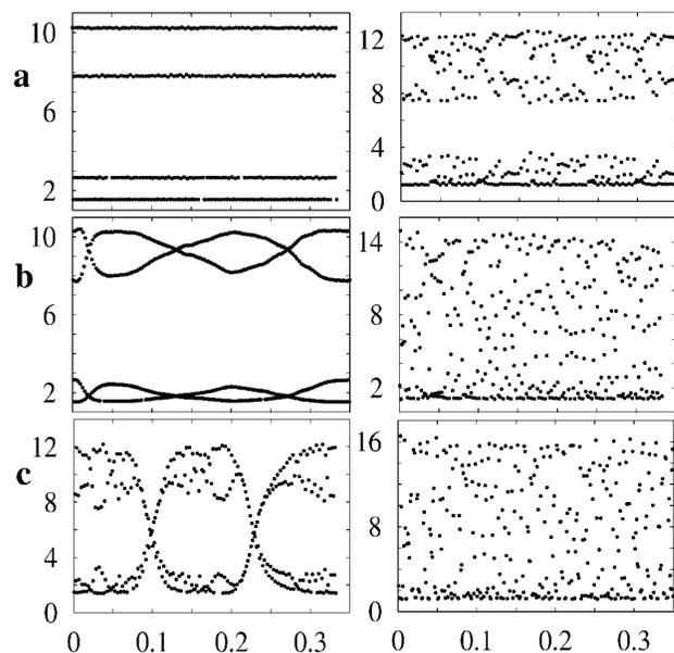
FIG. 2. Time series of  $c_z$  concentration maxima: (a)  $C = 4.30$ , (b)  $C = 4.42$ , and (c)  $C = 4.7$ . Left panels show the local dynamics at a point in the cells, while the right panels show the dynamics on the shock lines. Time is in units of thousands of spiral revolutions. In panels (b) and (c) the crossings of the  $c_z$  maxima reflect the passages through the observation point of  $\Omega_2$  or  $\Omega_1$  curves, respectively.
