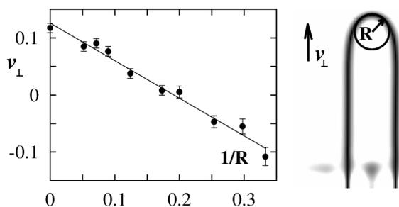
FIG. 3. Dependence of the domain propagation velocity,  $v_\perp$ , versus the curvature,  $1/R$ , of the tip for  $C = 4.30$ . A typical finger-shaped  $\Omega_2$  domain is shown in the right panel along with the inscribed circle used to determine  $R$ .
